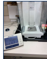
Left: Mettler Toledo model XS105DU with Max 120 g and d= 0.01mg (Scale 1)
